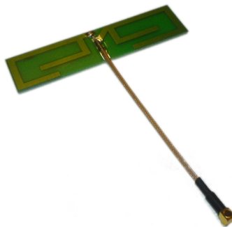
Figure 3.8: Picture of the antenna recommended by Acte, the reseller of the SocketModem EDGE
